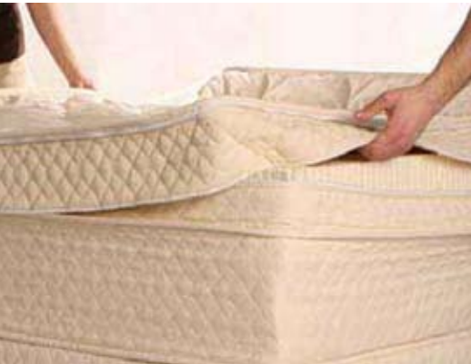
17. Place the top-cover over the layers of latex.
